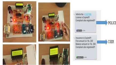
Our project contains RFID reader and RFID tags (vehicle insurance, driving license) whenever the tag is shown in front of the reader it will read the data from the tag, if it is valid it will display on LCD as valid otherwise the buzzer will buzz. Additionally, we are having alcohol sensor to identify whether the person is in drunk and drive or not. This process helps the user and police department to verify the documents of the vehicles whether the particular data is correct or not.
